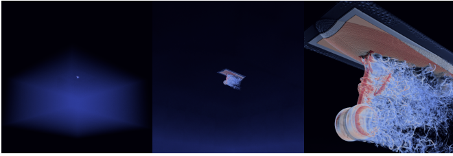
Fig. 2: Illustration of the spatial domains common to large unstructured data, here shown for the NASA Landing Gear AMR dataset. Elements throughout the simulation adapt in resolution to reduce memory consumption. From left to right, we progressively zoom in.
